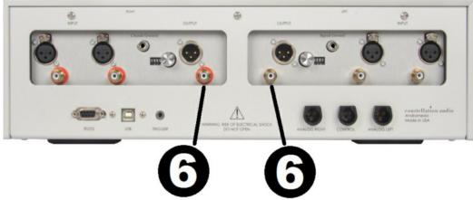
RCA unbalanced outputs are also supplied for preamplifers not equipped with XLR connections. When connecting to an amplifier, be sure to match the output to the correct channel on your amp. As you are looking at the back of the Andromeda, the output on the left side is for the right channel, and the output on the right is for the left channel. To remove an RCA plug, grasp it by the connector body and pull the plug out.
