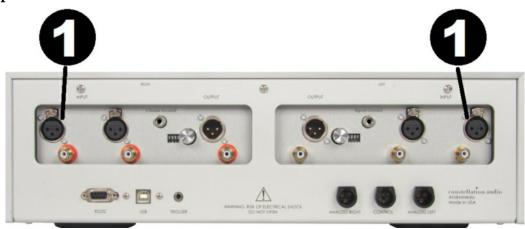
The XLR inputs farthest to each side of the back panel of the Andromeda are for use with MC cartridges. As you are looking at the rear panel, the left XLR inputs are for the right channel, the right inputs are for the left channel. These correspond with input MC-1. Use of XLR connections is recommended for the best possible audio quality. To remove an XLR plug, push on the tab above the jack and pull the plug out.
