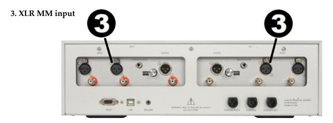
This XLR input is for use with MM cartridges. As you are looking at the rear panel, the left XLR inputs are for the right channel, the right inputs are for the left channel. These correspond with input MM. You may use either the XLR or RCA connection for input MM, but not both. Use of XLR connections is recommended for the best possible audio quality. To remove an XLR plug, push on the tab above the jack and pull the plug out.
