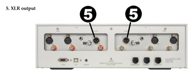
The inner XLR connections on the rear of the Andromeda are outputs. To remove an XLR plug, push on the tab on the connector body and pull the plug out. Be sure to match the output to the correct channel on your preamp. As you are looking at the back of the Andromeda, the output on the left side is for the right channel, the output on the right is for the left channel.
