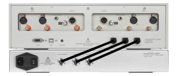
The Andromeda's separate power supply (bottom component in the picture above) must be connected to the Andromeda main chassis (top component in the picture above) as shown above before you plug the unit into a wall. Make sure the power switch on the power supply is in the off (O) position. The supplied cables are spiral-wrapped, gold-plated copper designed for aerospace use, and can handle up to 30 amps. Only these cables should be used between the power supply and the Andromeda.
