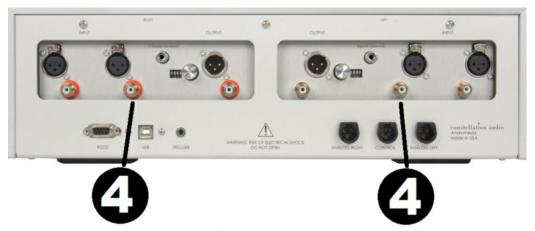
This unbalanced input is provided as a convenience for use with unbalanced signals from MM cartridges. These jacks correspond with input MM. You may use either the RCA or XLR connection for input MM, but not both. Whenever possible, we recommend using XLR connections instead. Connecting to an unbalanced source is handled in the same way an XLR balanced source. To remove an RCA plug, grasp the plug and pull it out. Do not pull on the cable.
