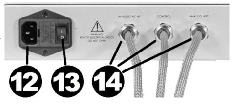
is flipped down. To power up the Andromeda, first flip this switch up, then either press the Standby button on the remote, or press the front of the touchscreen and hit the onscreen Power button or the middle button under the touchscreen.
